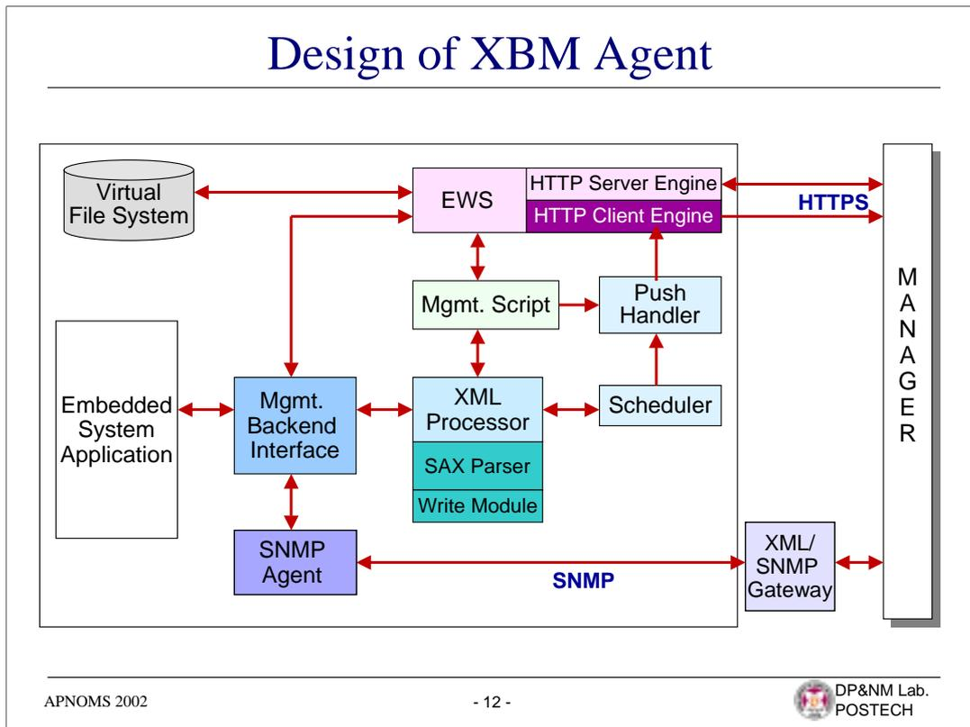
This slide illustrates the architecture of an XBM agent. The XBM agent includes an Embedded Web Server (EWS) [26] as a basic component. The components added to the EWS are the XML Handler having XML parser and SAX API, the Push Scheduler, and the HTTP Client Engine. In our previous work [3], we showed the use of DOM and XPath for handling the XML document. In the context of network management, DOM and XPath are good for processing XML document for accessing and filtering.
