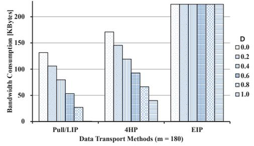
Fig. 5. Mathematical model based bandwidth consumption when  $m = 180$  and  $D$  changed from 0.0 to 1.0.
