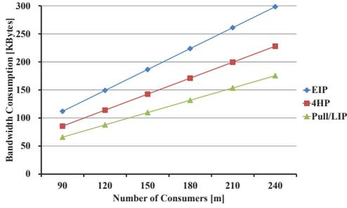
Fig. 3. Bandwidth consumption (y) versus number of data consumers (x) when  $D = 0$  and  $m$  changed from 90 to 240.
