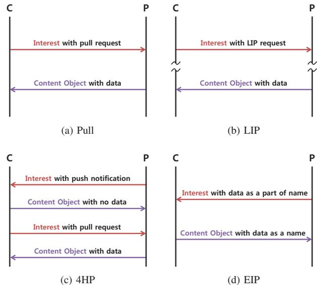
Fig. 1. Flows of Interest and Content Object packets in four data transport methods of CCN: Pull, Long-lived Interest Push (LIP), 4-way Handshake Push (4HP), and Embedded Interest Push (EIP).
