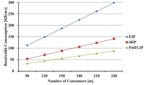
Fig. 4. Bandwidth consumption (y) versus number of data consumers (x) when  $D = 0.5$  and  $m$  changed from 90 to 240.
