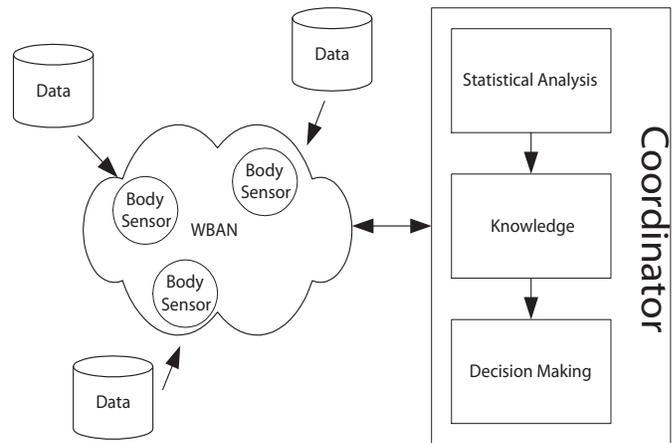
Fig. 1. WBAN system architecture
