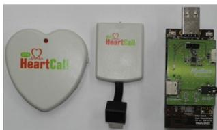
Figure 3. Uheart ECG sensor and Hybus Wireless Sensor Base
