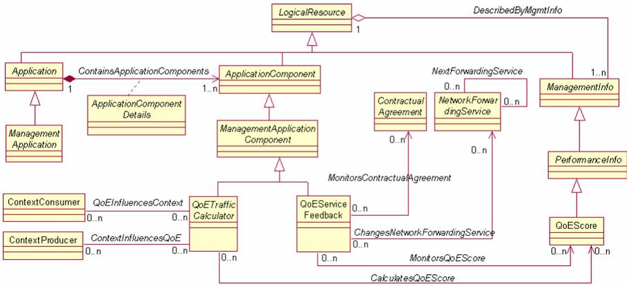
Fig. 3. QoE Control Loop - Model View
